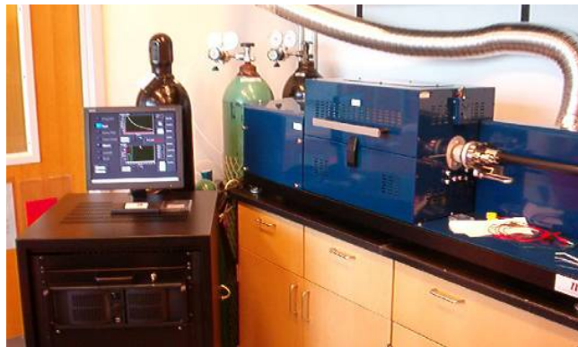
Figure 5.4 First Nano Easy Furnace used to anneal graphene oxide CNT composite samples.
