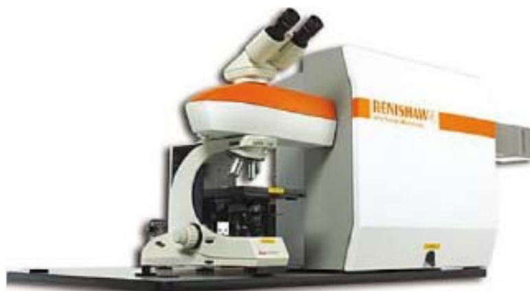
Figure 3.17 Renishaw Invia Raman Microscope with a 488 nm Ar + laser. Taken from reference [99].
